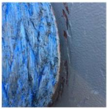
• Removing or adapting the Chafe Guard to fit the bollard at port will cause the Chafe guard to be less effective and easily damaged. This will decrease the protection of the rope.
