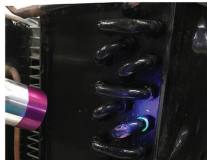
Refrigerant leaks in the system glow brightly when exposed to UV light from SuperBright UV-LED Torch.
