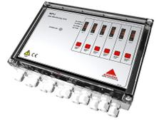
The connected detector continuously measures the gas concentration and provides an analogue signal to the central unit. Alarms are indicated in three levels by a yellow and two red LEDs that indicate low (Alarm C), medium (Alarm B) and high (Alarm A) gas concentration, the respective LED lights up and the corresponding relay switches. If the alarm delay selected flashes each LED in the selected delay time, then the LED turns to steady and the relay contact switches.
