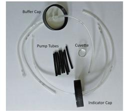
Generally, both pump tubes should be replaced annually. Spare cap assemblies for both the buffer and the indicator are supplied and can be replaced when needed.
